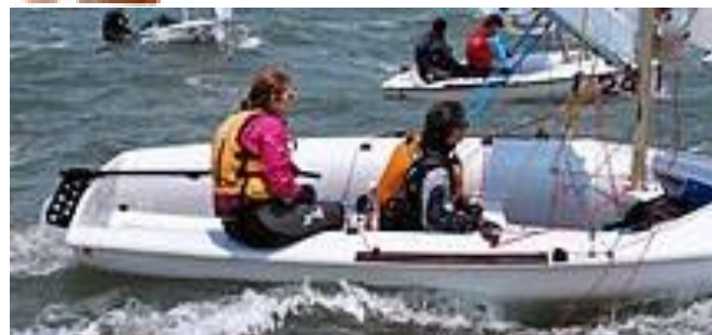
Using a tiller (the black rod) with tiller extension on a 420 sailing dinghy
