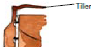
Simple tiller on a wooden boat
